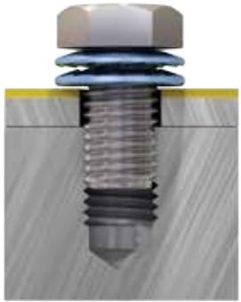
A pair of Nord-Lock X-series washers has cams on one side and radial teeth on the opposite side to secure the bolted joint with tension instead of friction. The conical shape creates an elastic reserve in the bolted joint to compensate for the loss of preload and prevent slackening.
